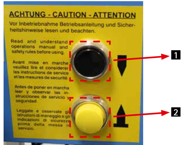
Fig. 37: Manually operated valve and momentary switch
