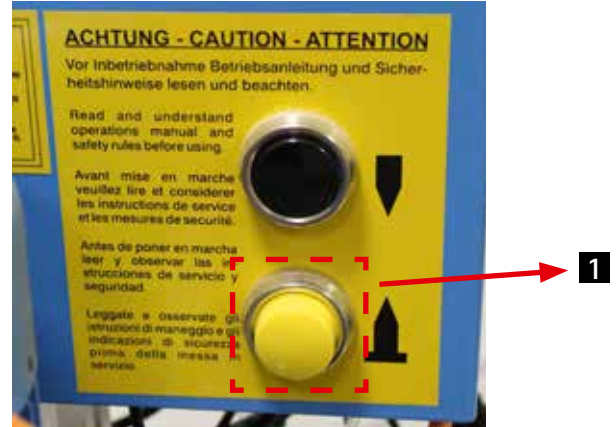
Fig. 27: Yellow button: Releasing the hold-down clamps
