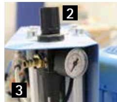
Fig. 7: Compressed air connection
