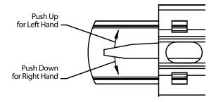
To disconnect drawer member, first extend the slide fully and then lift up the left hand side disconnect lever and push down the right hand side disconnect lever and pull the drawer member out.
