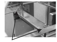
Re-install nuts on top for clearance
