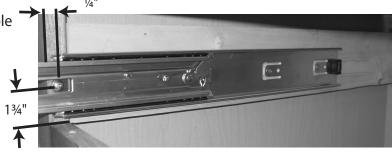
**Step 4.** Using the 5mm Allen wrench, and 10mm wrench, remove the board and front support from the friction slide units.
